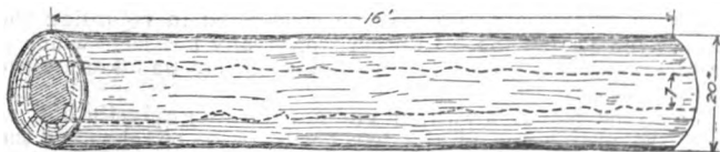
FIG. 4.—Deduction for defect caused by center or circular rot
