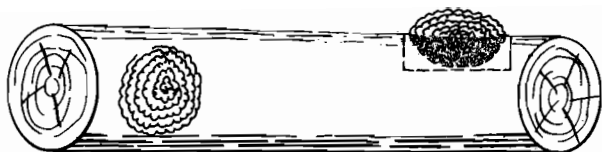
Figure 33. -Burls-combination pie-cut and length-deduction method.
